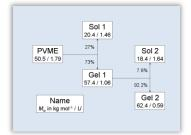
By the choice of the fractionation parameters (temperature, compositions) the "cut" through the molecular mass distribution can be varied. Narrow molecular mass distributions can be achieved by repeated fractionation.
